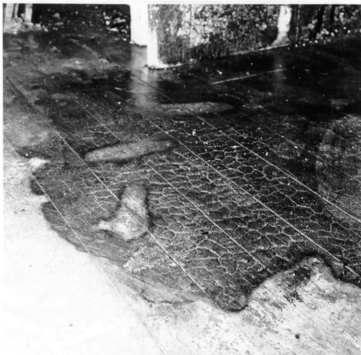
Above: These burn patterns were revealed after the debris was removed and the floor washed. This pointed to an arson attack and the early arrest of the offender. Unfortunately the company never recovered and closed down soon after.
