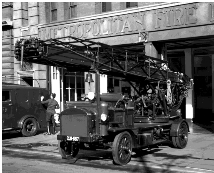
The Morris Magirus turntable ladder outside the old FS2 in William Street. It was still in service in the 1950's. During the war years, American soldiers would heckle the crews about the old fashioned ladders and solid rubber tyred wheels.
