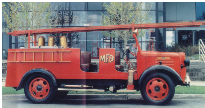
Above, "Bedford Hose Carriage Car 75" Designed and built by the MFB Workshops. Later fitted with a 150 gallon first aid tank, served at Greensborough and Deer Park, 44D (Pictured below)
